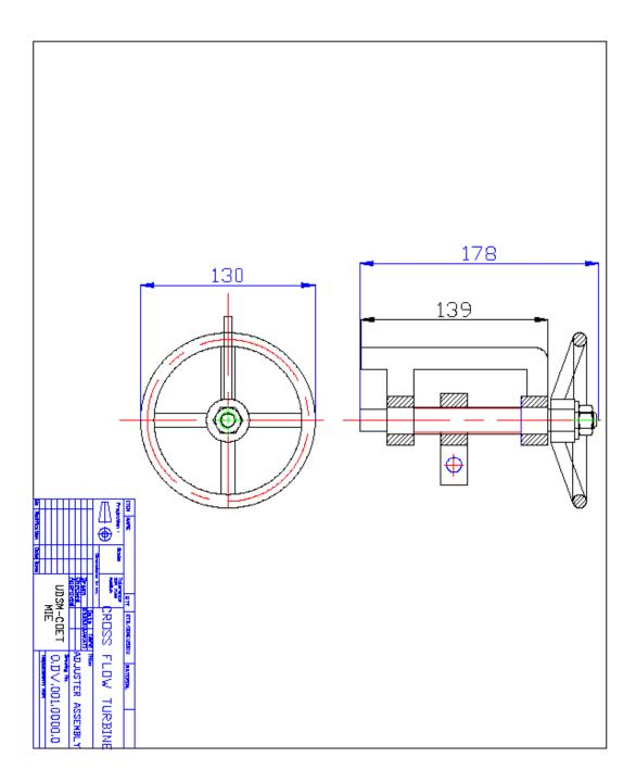
Figure A-2: Adjuster sub assembly, Source: Wakati (2010)
