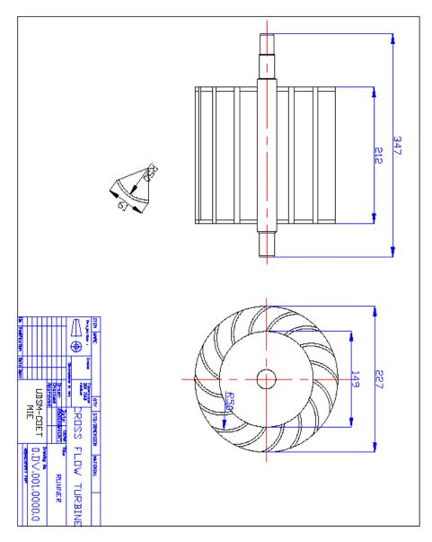
Figure A-5: Crossflow turbine Runner Source: Wakati (2010)
