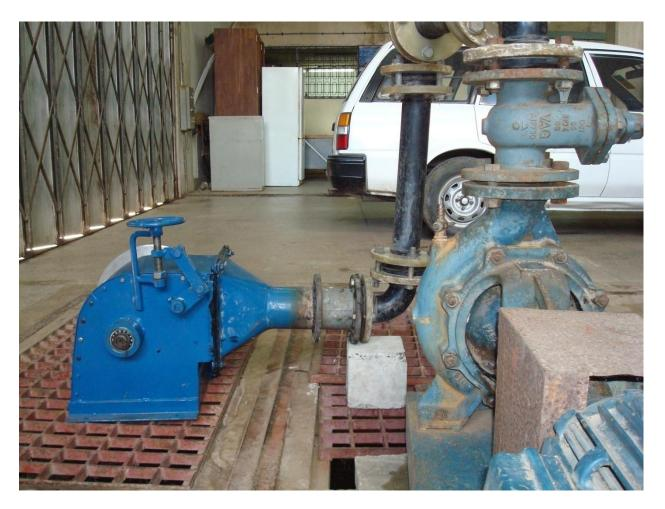
Figure 4. 1 Cross flow turbine testing (Wakati (2010)
