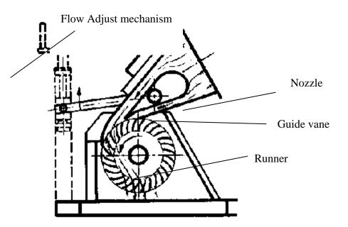
Figure 3.1: Schematic diagram of Cross flow Turbine (adopted from Wakati, 2010)
